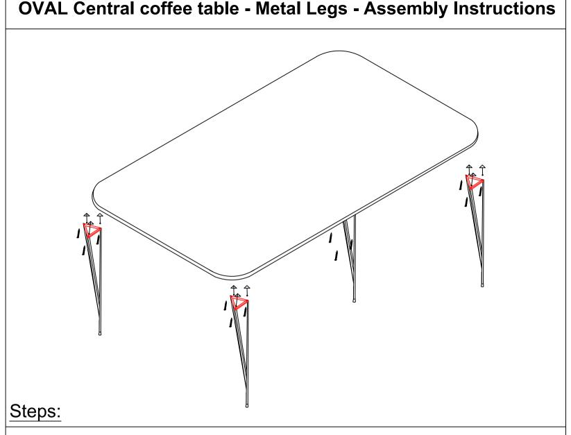
There are 1 big size table tray, 4 Long height Metal legs Position the tray on flat surface. Attach the tray to the legs with the mounting screws to the pre-drill holes marked on the tray.
